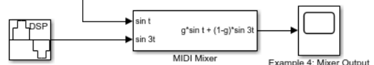
Example 4: Use the MIDI control surface to control the mix as you combine two signals into one
