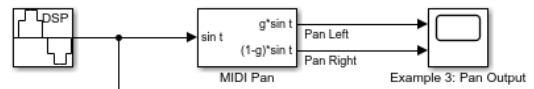
Example 3: Use the MIDI control surface to control the relative amplitudes as you split a single signal into two
